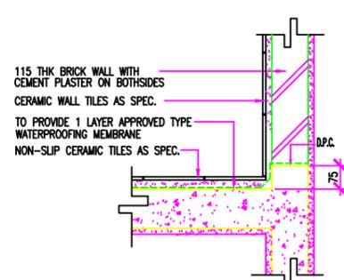
TYPICAL FLOOR & WALL DETAIL FOR WET AREA
